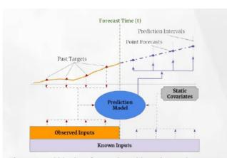
Figure 4. Multi-horizon forecasting with static covariates, past observed and a priori-known future time-dependent inputs
